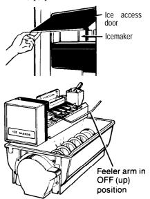
When water supply has been connected to icemaker, move feeler arm to ON (down) position.
